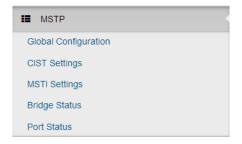
The Spanning Tree Protocol (STP) is a network protocol that builds a logical loop-free topology for Ethernet networks. The basic function of STP is to prevent bridge loops and the broadcast radiation that results from them. Spanning tree also allows a network design to include spare (redundant) links to provide automatic backup paths if an active link fails. This is done without the danger of bridge loops, or the need for manual enabling or disabling of these backup links.
